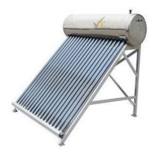
The total system is installed in the roof top and on one side of the solar tank, cold water is connected and from the other side, piping is done upto bathroom and kitchen. The requirement at the site is basically shadow free area (as mentioned) facing south and the bottom of the overhead tank to be at a minimum of 5 feet height from the roof level.
